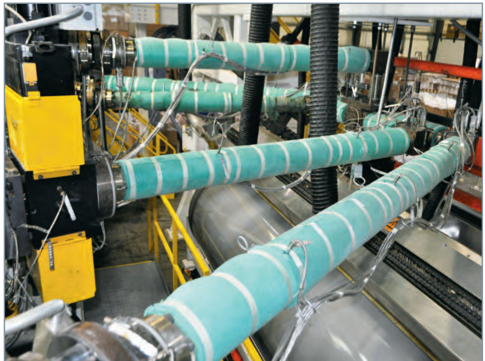
CONSISTENT TEMPERATURE OVER GREAT LENGTHS. SmartHeat™ coating from Nordson Xaloy enables extrusion melt pipes and adaptors to deliver more uniform melt than in systems with conventional heater bands. (Photo courtesy of Paragon Films, Inc.)
