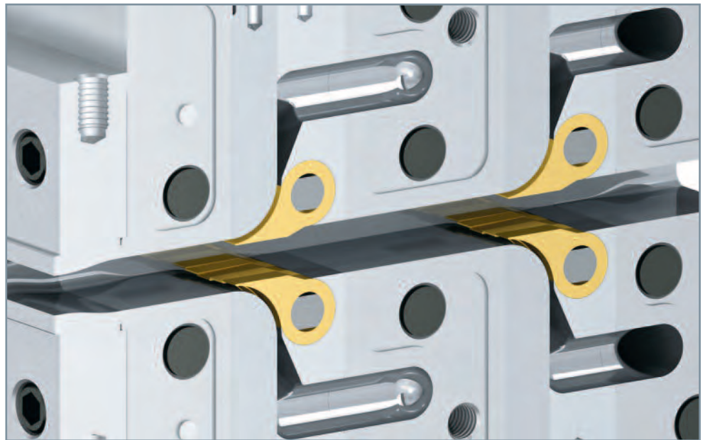
SPEED AND PRECISION. In generalized schematic of new tuning insert for Ultraflow™ I feedblock from Nordson Extrusion Dies Industries, polymer flow for a five-layer structure is from right to left. Core layer polymer enters flow channel from far right. Next layer enters from ports at top and bottom, and its thickness profile is determined by bronze-colored flow-adjusting components. Entry of skin layer follows, again profiled by flow adjusters. Each adjuster is made up of multiple and adjustable segments.
