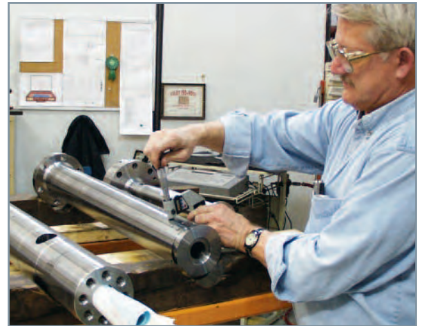
INSPECTION OF NEW COMPONENTS is the final stage in Nordson XALOY's process for the design, engineering, and production of precision screws and barrels. Nordson XALOY draws on huge databases of screw designs and resin rheologies and operates two rheological laboratories for customers.
